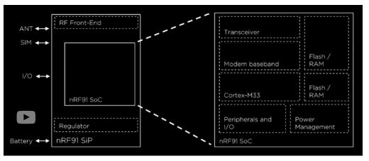
The nRF91 Series SiP has been jointly developed by Nordic's experienced cellular design team in Finland and its low power wireless experts in Norway. The SiP comprises RF front-end, nRF91 Series SoC, and regulator
