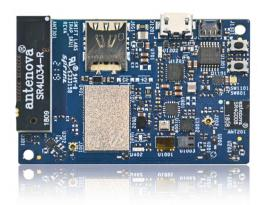
offers an accelerometer and temperature sensor as standard, multimode LTE-M/ NB-IoT capabilities, GPS and a powerful Arm Cortex-M33 application processor.
