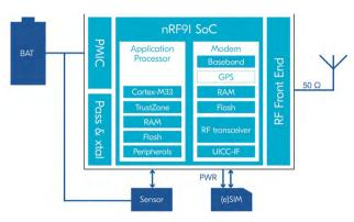
Through high integration and precertification for global operation, the nRF9160 solves the complex wireless design challenges arising when employing cellular technology requiring just an external battery, SIM, antenna and sensors
