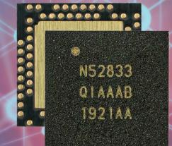
TX power: +8 dBm Concurrent multiprotocol 64 MHz Arm Cortex-M4 with FPU
