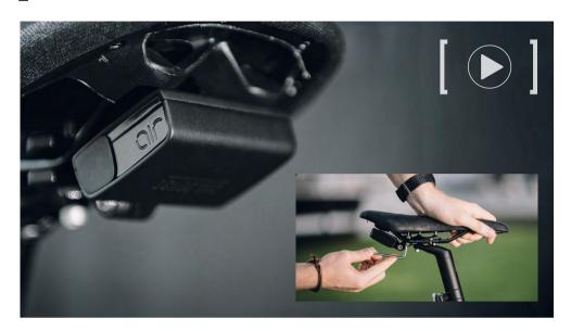
AIR will not only protect the bike, it will also protect its rider, identifying if the bike's been involved in a crash and sending an SMS with the precise location to the rider's assigned contact.
