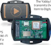
continuous location tracking, traceability, loss/theft prevention and movement/impact detection of assets that frequently move between indoor and outdoor locations. The GNSS technology also offers assistance for quicker time-to-first-fix (TTFF) with the data downloaded to the device via the cellular network. When no GNSS or Wi-Fi signal is available, cellular IoT connectivity enables location/position monitoring of assets.
