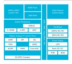
The nRF52811 supports Bluetooth 5.2, 802.15.4, Thread and 2.4 GHz proprietary. The nRF52811 offers a good option for a network processor and when paired with a companion microprocessor is a high value proposition for smart home gateway and router applications
