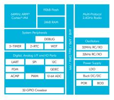
The nRF52810 supports Bluetooth 5.2 and 2.4 GHz proprietary. The Soc forms the ideal compromise between advanced performance, functionality and cost. It offers a good option for a network processor and when paired with a companion microprocessor
